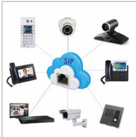
Figure 1: SIP Unified Communication Network
